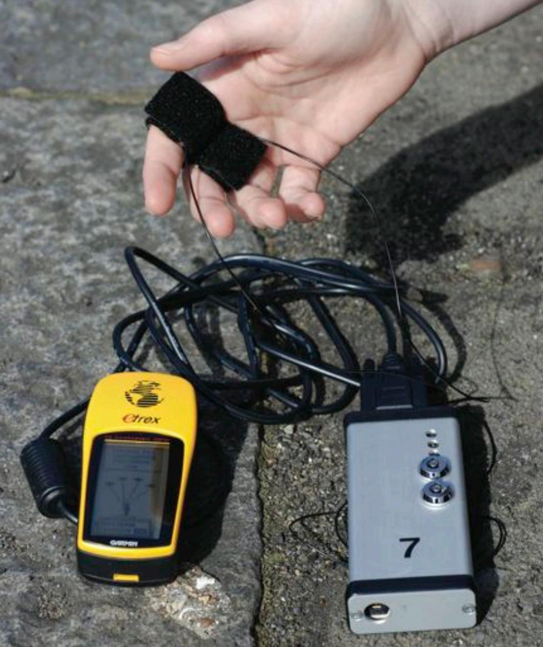
*The Bio Mapping device: GPS – left, fingercuffs – top and data logger on the right.*
